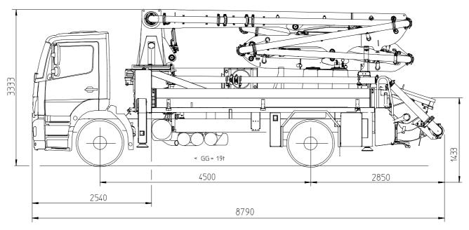
Note: Standard version. Dimensions and weights depend on truck and pump model.
