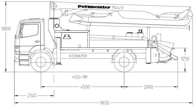
Note: Standard version. Dimensions and weights depend on truck and pump model. Dimensions in mm, MB-Axor 1828 as example
