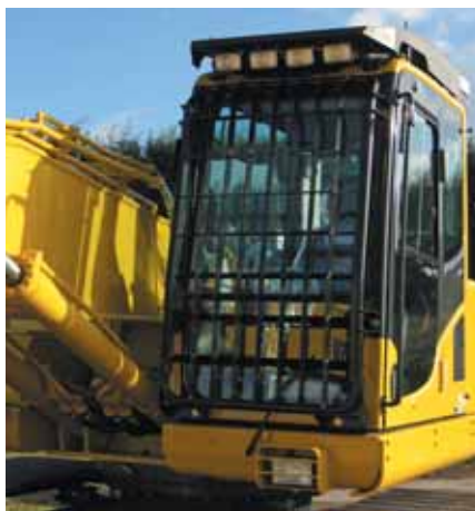
The demolition specification operator cabin includes ISO 10262 Level 2 certified FOPS (Falling Object Protection System), safety glass roof window with wash wipe system and controls for extra hydraulic functions.
