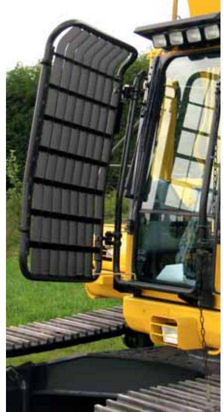
The FOPS guard system includes a side hinged front guard, allowing the operator easy access for periodic windscreen cleaning.
