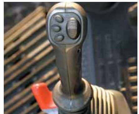
Joysticks with proportional control button for attachments.
