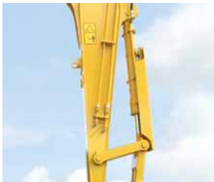
The attachment cylinder guard is one of many safety features on high reach excavators, along with a hinged type front FOPS guard, safety valves, a rear view camera and working range limit warning device.
