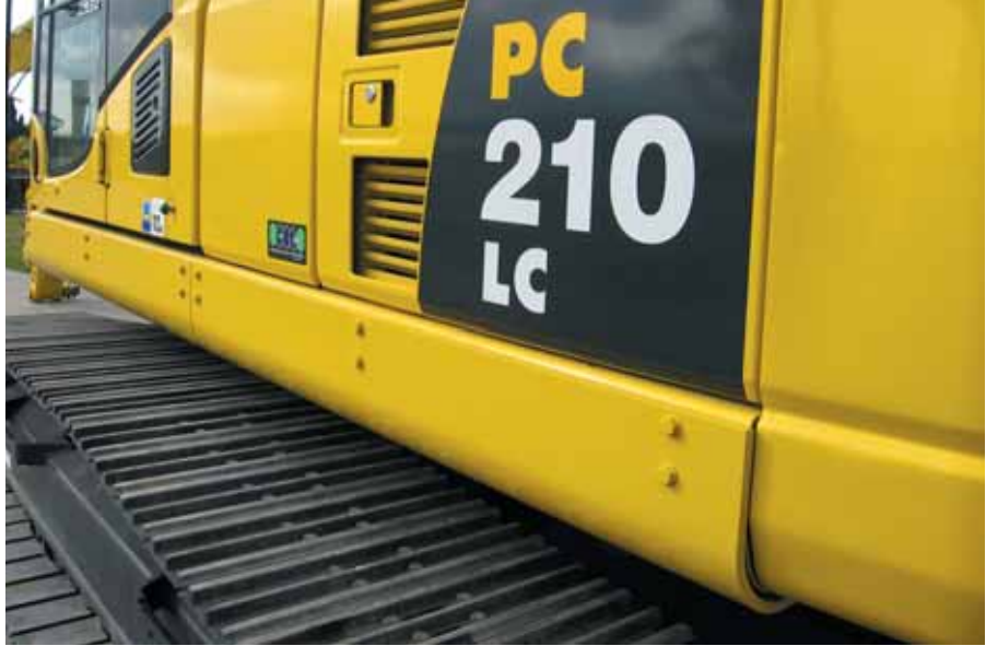
Bolted on extra-heavy duty side protections are fitted to either side of the upper structure and can be easily removed for maintenance or transport.
