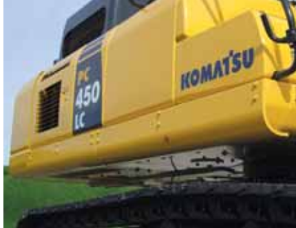
Standard heavy duty bolt-on side guards and under covers protect all the machine's state-of-the-art systems from damage.
